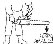
In case the brake is not effective, ask our dealer for inspection and repairs. If the engine keeps rotating at high speed with the brake engaged, the clutch will overheat causing trouble. When the brake engages during operation, immediately release the throttle trigger to stop the engine.
