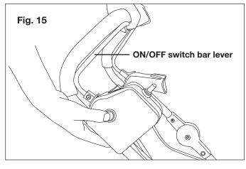
To power off, release your grip on the ON/OFF switch bar lever.
