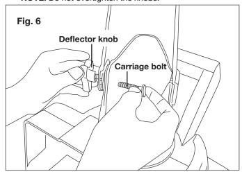
4. Raise or lower the chute deflector by loosening and tightening the deflector knobs to achieve the desired snow stream height.
