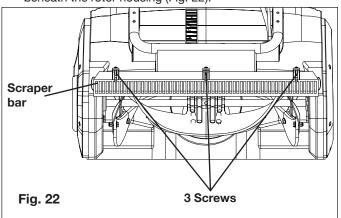
Detach the worn scraper bar from the snow blower by removing the 3 screws that hold it in place (Fig. 23).
