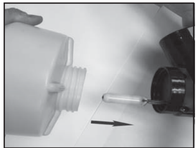
12. Thread jar back onto fogger.
