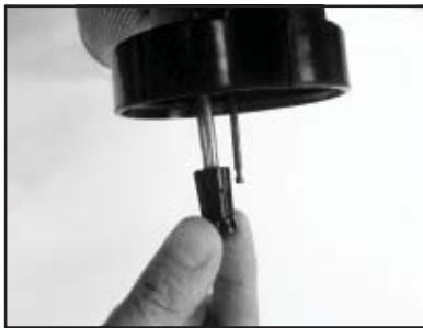
4. Unthread piston assembly.
