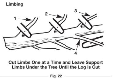
**NOTE:** If possible, the log should be supported so that the end to be cut off is not resting on the ground. The best way to hold a log while bucking is to use a sawhorse. When this is not possible, the log should be raised and supported by the limb stumps or by using supporting logs. Be sure the log being cut is securely supported.
