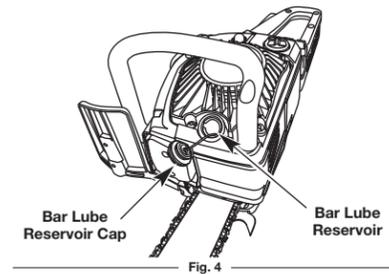
Fill the bar lube reservoir each time the fuel tank is filled. Only use bar and chain oil that is formulated to perform over a wide range of temperatures with no diluting required in the bar lube reservoir. Do not use motor oil or any other petroleum-based oil.
