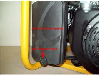
The Air Cleaner is located to the left of the recoil starter assembly.
