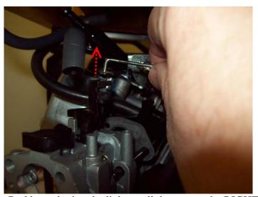
Remove the Pulling Rod by swinging the linkage all the way to the RIGHT and pulling up on the rod.
