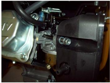
Attach the 10mm Nut to the OUTSIDE of the Air Cleaner Housing.
