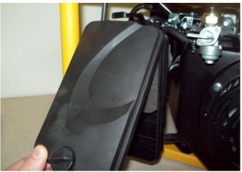
Remove the cover by unscrewing the knob located near the bottom of the cover. Pull up on the bottom and allow the top to clear the two tabs holding it in place. Then remove the cover and set it aside.
