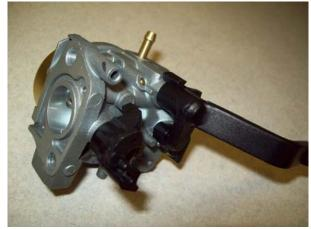
When attaching the Choke Lever, install it over the top of the Post molded into the Carburetor and make sure the Pin of the Choke Lever seats in the slot on the Linkage.
