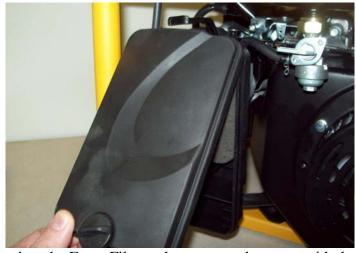
Reinstall the Grate...then the Foam Filter...then engage the cover with the two tabs on the top of the housing...then swing the cover down into position and tighten the knob to secure the cover.
