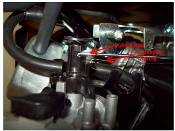
Remove the regulating spring from the Carburetor linkage and allow the spring to dangle free for later reassembly.
