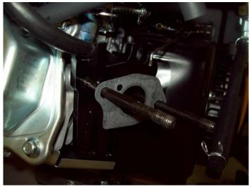
There is a Gasket BETWEEN the Carburetor and the Connecting Block. Remove it and set it aside for reassembly later on.
