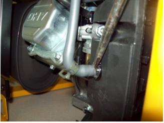
On the LEFT side of the Air Cleaner housing you will see a rubber hose. Remove the clamp with pliers and slide it up the tube. Insert a flat screwdriver blade between the hose and the housing and wiggle the hose away from the plastic nipple. The screwdriver will help break the seal between the hose and the nipple.
