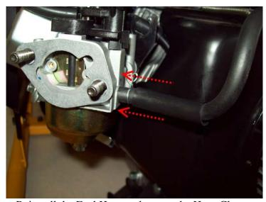
Reinstall the Fuel Hose and secure the Hose Clamp.
