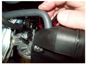
Push the hose from the OHV Cover back down into the Air Cleaner Housing.
