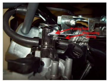
Reattach the Pulling Rod and Regulating Spring on to the Carburetor Linkage.
