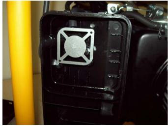
Remove the metal grate from the Air Cleaner housing. It is held in position by two plastic pins. Pull he grate straight off the pins and set it aside.
