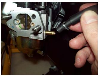
If you are removing the Carburetor, disconnect the fuel hose by releasing the hose clamp and sliding it back on the hose. (NOTE: Be sure the fuel valve is turned to the OFF position under the gas tank.) Remove the hose by pulling it away from the carburetor.
