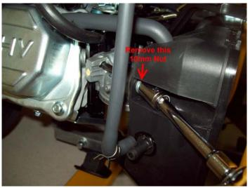
Remove the 10mm nut located above the vent hose you just removed.
