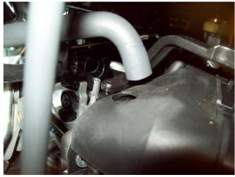
There is an air duct that goes from the Air Cleaner to the OHV cover on the engine. Remove this air duct from the Air Cleaner by pulling up on it. It is a friction fit. There are no clamps. Remove the Air Cleaner to expose the carburetor.
