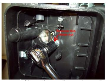
Under the grate you will see a 10mm nut. Remove the nut and set it aside.
