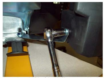
Locate the 10mm screw on the underside of the Air Cleaner assembly. It secures a bracket that goes from the engine block to the Air Cleaner. Remove the screw and set it aside.
