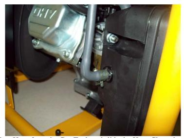
Reinstall the Vent Hose from the Gas Tank and slide the Hose Clamp back into position.
