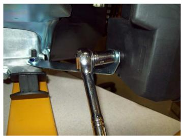
Reinstall the 10mm Bolt through the bracket and into the Air Cleaner Housing.
