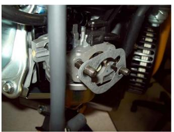
Note there is a gasket BETWEEN the Air Cleaner and the Carburetor.
