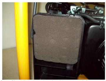
Next, remove the foam filter element and set it aside. (Note: It is normal for the filter to feel slightly oily.)
