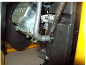
On the LEFT side of the Air Cleaner housing you will see a rubber hose. Remove the clamp with pliers and slide it up the tube. Insert a flat screwdriver blade between the hose and the housing and wiggle the hose away from the plastic nipple. The screwdriver will help break the seal between the hose and the nipple.
