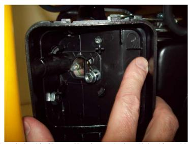
Attach the Air Cleaner Housing and reinstall the 10mm Nut.
