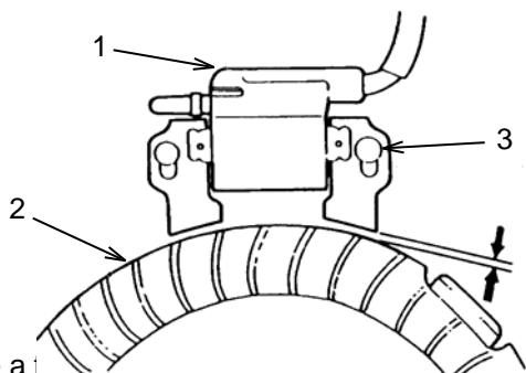
Use a feeler gauge between the ignition coil (1) and the flywheel (2). The clearance should be 0.4 – 0.6mm. If the clearance is out of the acceptable range, loosen screws (3) and move the coil so that the clearance is within range. Retighten the screws.
