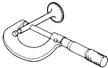
Use a micrometer to measure the outside diameter of the valve stem. Refer to the following table.
