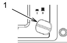
The panel light (1) is held to the panel with hot melt glue. Disconnect the panel light from the
