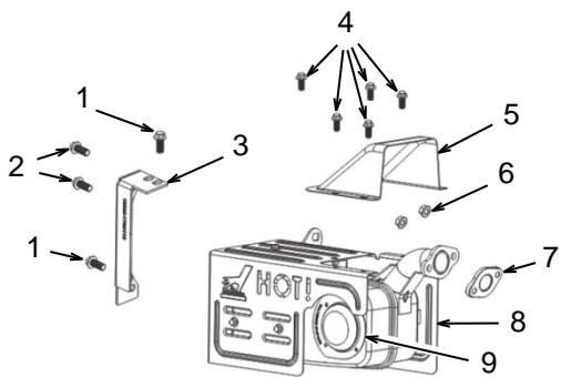
Remove bolts (1) and (2) and remove bracket (3). Remove bolts (4) and cover (5). Remove nuts (6) and lift muffler (8) off of the mounting studs. Discard used gasket (7). Removing the cover from the muffler is not recommended. Reinstall in reverse order using a new gasket (7). To service the spark arrestor, refer to Spark Arrestor – Inspect/Clean/Replace.
