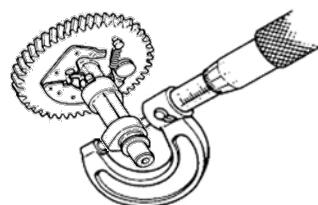
Inspect the camshaft for damage or abnormal wear. Measure the lift on the camshaft lobes. The acceptable limit for the lift is shown in the table below. If the lift is out of the acceptable range, replace the camshaft.
