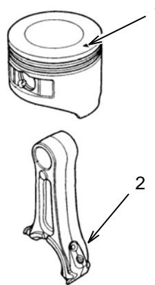
Place the connecting rod into the piston so that the longer side of the rod (2) is aligned with the mark on the piston head (1). Insert through one side of the piston, through the connecting rod, and then through the other side of the piston.
