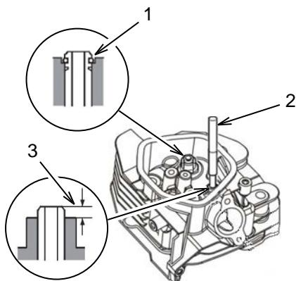
Install the new valve guides from the valve spring side of the cylinder head. Use the valve guide driver (2) to drive the exhaust valve guide in until the clip is fully seated (1). Drive the intake valve guide in until the top of the valve guide extends 1mm above the cylinder head (3). After installation check each valve guide for
