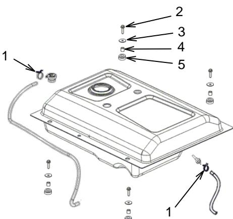
Remove hose clamps (1) and fuel lines from the rollover sensor and the fuel filter. Remove all
