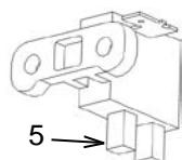
Check the length of the brushes (5). If the length is 6mm or less, replace the brush. To remove the brush, remove bolt (1) and disconnect the leads. To reinstall, connect the red lead to the "+" terminal, the white lead to the "-" terminal, then use bolt (1) to secure the new brush.
