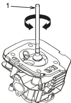
Apply lapping compound to the valve face and insert the valve into the cylinder head. Use a valve lapping tool (1) to finish surfacing the valve and valve seat. Remove any remaining compounds before assembling the cylinder head. Make sure that the pushrods are firmly seated in the lifters. After assembly, follow the Engine Valve Lash – Adjust and the Cylinder Pressure – Check procedures to ensure a proper assembly.
