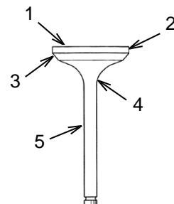
Check the valves for damage. Check the valve head (1), valve margin (2), and valve face (3) for damaged or burnt areas. Check the valve neck (4) for unusual wear. Check the valve stem (5) for wear, scoring, or bends. If any damage is found, replace the valve.
