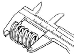
Check the free length of the valve spring. The normal free length is 34mm. If the free length is 32.5mm or less, replace the spring.
