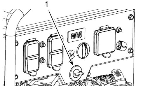
The fuel valve (1) can be accessed without removing the control panel. To remove the fuel valve, drain the fuel from the fuel tank into an appropriate container. Start the engine and let the engine run out of fuel. Turn the generator switch to the off "0" position.
