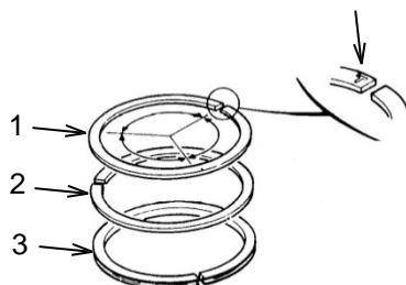
The piston rings have a mark next to the gap. Use a ring puller to install the rings with the mark facing toward the top of the piston. Make sure that you install the rings in the proper grooves, with the oil ring (3) in the lowest groove, the second ring (2) in the middle groove, and the top ring (1) in the groove closest to the head of the piston. The top ring is chrome plated. Make sure that the rings will move freely in the ring groove.
