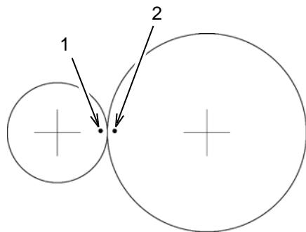
The crankshaft and cam shaft both have alignment marks on the gear face. Use these marks to align the gears during assembly. When aligning the marks, make sure that the piston is at the top dead center position.
