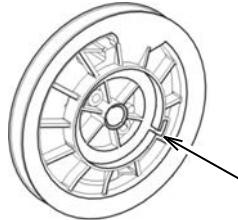
Place the outside hook of the recoil starter spring in the groove of the recoil starter pulley and hold the pulley in place.
