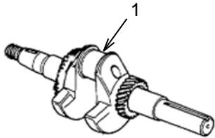
Check the diameter of the crankshaft journal (1). A normal diameter is 30.190mm. If the diameter is 30.175mm or less, replace the crankshaft.
