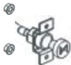
The choke is held to the rear of the panel with 7mm nuts. Remove the choke knob and cable from the front of the panel, and remove the nuts that hold the choke to the panel. Remove the choke control from the rear of the panel. Reinstall in reverse order.
