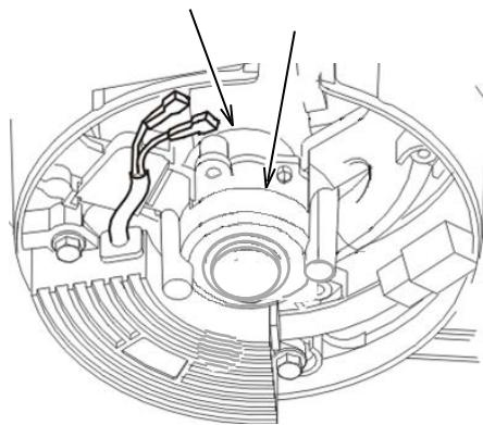
Remove the brush. Use an Ohmmeter or multimeter to measure the resistance of the collector ring at the points shown. The resistance should be  $58.5 \pm 10\Omega$  at  $25^\circ\text{C}$ . If the resistance is out of tolerance, clean the collector ring and retest. Replace the generator if necessary.
