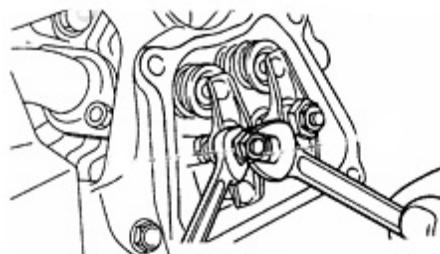
Loosen the locking nut. Turn the adjustment nut clockwise to decrease the gap. Turn the
