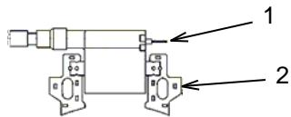
Measure the resistance of the primary coil by touching one lead of an Ohmmeter to the primary terminal (1) and touching the other lead to the metal frame (2). If the resistance is not in the 0.8 – 1.0Ω range, replace the coil.
