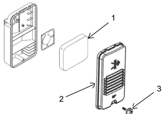
Remove the air filter cover bolt (3) and remove the air filter cover (2). Make sure that the air filter (1) is clean and not damaged. If the air filter is
