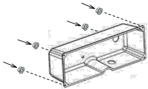
Place the front of the control panel on a surface that will protect the panel from damage. Remove the four 7mm nuts from the back of the control panel housing and carefully separate the housing from the front panel.
