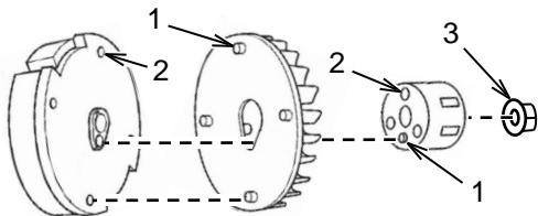
Align the positioning pins (1) on the starter cup and both sides of the impeller with the holes (2) in the starter cup and flywheel. Place the assembly on the crankshaft. Secure the assembly to the crankshaft with nut (3). Tighten the nut to  $95\pm4$  N·m ( $70\pm3$  lbft).
