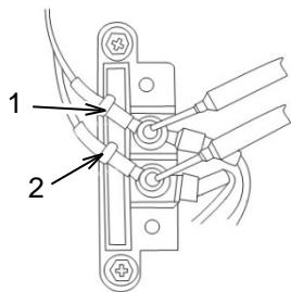
On the terminal block, use an Ohmmeter or multimeter to measure the resistance of the main winding. Place the meter across the white wire (1) and the brown wire (2). The resistance should be  $0.35 \pm 10\Omega$  at  $25^\circ\text{C}$ . If the resistance is out of tolerance, replace the generator. Measure the resistance from the wires to ground. The resistance should be infinite. If the resistance is not infinite, replace the generator.
