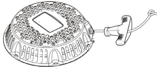
Wrap the cord around the pulley. Pull lightly on the cord and push the end of the cord through the housing. Then push the end of the cord through the handle. Tie a knot in the end of the cord and let the spring pull the handle back to the housing. Pull lightly to make sure that the assembly is working properly.
