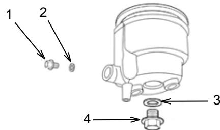
Install drain plug (1) and gasket (2) into the float chamber. Set the float chamber in place so that the drain bolt can be accessed from outside the unit. Install gasket (3) and bolt (4) to hold the float chamber in place. Reinstall the carburetor. After starting the unit, check for leakage. Bring the engine to the normal operating temperature and adjust the pilot screw to bring the engine to the proper idle speed.
