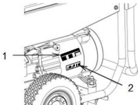
Cat portable generators are identified with model numbers, serial numbers, and with performance specification numbers. The model number and performance specifications are located on the ratings plate (1). The serial number is located on the serial number plate (2).
