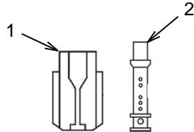
Inspect main fuel jet (1) and main fuel nozzle (2). If worn, replace.
