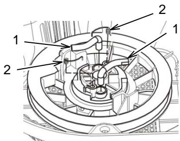
Set the starter drive cams (1) on the recoil starter pulley, and install the return springs (2) on the pulley and hook them on the side of the drive cams.
