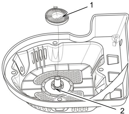
Place the inside hook (1) of the recoil starter spring in the groove (2) of the recoil starter case and set the recoil starter spring into the case. Hold the spring in place.
