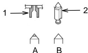
Check the float valve seat (1) and float valve (2) for wear. Figure A shows a worn float valve that needs replaced. Figure B shows a float valve that can be reused.
