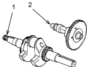
Inspect the gears on and the crankshaft (1) and the camshaft (2). If the gears are worn or any teeth are broken, replace the gear. Check the engagement of the gears. If the gears fit together too loosely the engine will run louder than normal. It is recommended that you replace the gears if the engagement is loose. If you must replace the gears or shafts, replacing them one at a time will lessen the chance of assembling them incorrectly.
