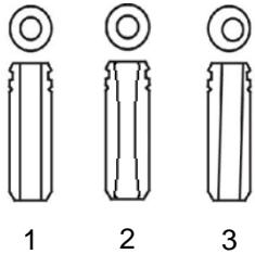
Check the valve guide bore. Insert the valve and make sure that it moves smoothly through the bore without any wobble. Figure 1 shows a good valve guide. Figure 2 shows a valve guide with abnormal wear that would allow the valve to wobble. The valve head could eventually break off and fall into the combustion chamber, damaging the engine. This valve guide must be reamed or replaced. Figure 3 shows a valve guide with a bore that is not centered. This valve guide must be replaced.
