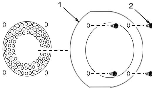
Remove screws (2). Remove spark arrestor (1) Check the spark arrestor. Carefully clean the spark arrestor with a soft wire brush. If the spark arrestor is damaged, replace the spark arrestor.
