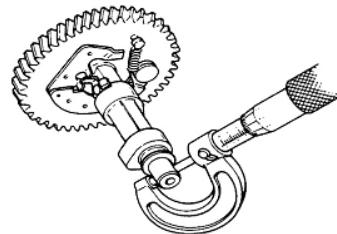
Measure the outside diameter of the camshaft. The normal diameter is 13.984mm. If the diameter is 13.916mm or less, replace the camshaft.
