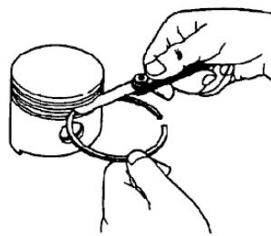
Measure the ring clearance, as shown. Normal clearance is between 0.015 and 0.045mm. If the clearance is 0.15mm or more, replace the piston.
