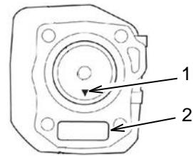
Coat the piston, rings, and cylinder wall with engine oil. Use a ring compressor to push in the rings and insert the piston into the cylinder. Make sure that the mark on the piston head (1) aligns with the lifter mark (2) on the crankcase. Use a piston driver to push the piston out of the ring compressor and into the cylinder.
