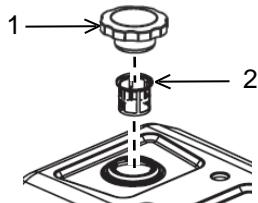
Wipe off the fuel cap (1) and surrounding area before removing the fuel cap. Wiping off the fuel cap and surrounding area before removing the fuel cap helps to reduce the amount of contaminants allowed into the fuel system.
