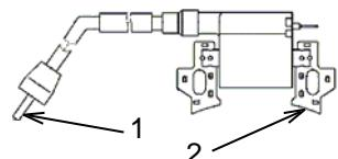
Measure the resistance of the secondary coil by touching one lead of an Ohmmeter to the spark plug wire (1) and touching the other lead to the
