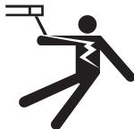
**When triggering, the electrode and drive mechanism are electrically "hot" relative to work and ground and remain "hot" for several seconds after the gun trigger is released.**
