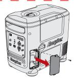
**1.** Setup the Battery: Remove the Battery Access Panel from the unit by unscrewing the screw at the top and releasing the panel.
