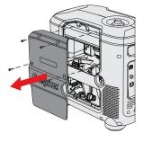
**4.** Remove the main engine access panel from the unit by unscrewing the (4) screws at the top and middle of the unit.
