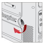
4. Close the fuel valve by turning it to "Off".
