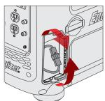
2. Connect the Battery: locate and connect the loose connectors from the battery wiring harness and the main wiring harness. The battery is now connected to the unit.
