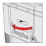
**3.** Turn choke to fully "Closed" position. Leave the choke in the "Open" position if the generator is still warm from recent use, or if the air temperature is higher than 50°F (10°C).
