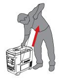
**5.** Pull Recoil handle until engine starts. Several pulls may be required until engine starts. Do not release the pull cord at the end of a pull, this will damage the recoil assembly. Bring the pull handle back down to the unit by hand.
