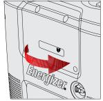
**6.** Once the generator has started, wait at least 30 seconds for it to warm up, and then you may slowly open the choke lever until it is fully open.
