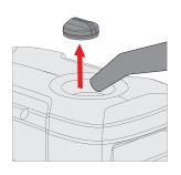
**9.** Remove the fuel cap, exposing the fuel tank. Be sure not to allow any dust or debris near the engine during this time. Pour 91 octane unleaded gasoline into fuel tank, add Ethanol Shield $^{\text{TM}}$  to fuel tank as directed on bottle, and replace the fuel cap.
