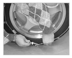
On the outside of the tire, thread the cable with bushings through the end hook for initial mounting. Grasp the outside side cable with both hands and pull it towards you. This will create as much slacks possible. Then make the outside connection in the same manner.
