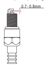
Standard Spark Plug: E6TC/E6RTC/BPR6HS
