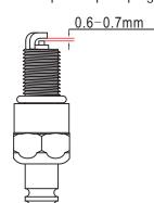
Standard Spark Plug: E6TC/E6RTC/BPR6HS
