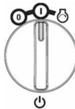
Turn the generator switch to the start position "S" and hold until the engine starts (no more than 5 seconds). Releasing the switch automatically returns it to the on "I" position. To turn off the generator, turn the generator switch to the off "0" position.
