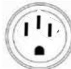
The 120/240 VAC outlet is protected against overload by a 48 Amp double pole circuit breaker. Use a NEMA L14-50 plug with this receptacle. Use the receptacle to power a 120 VAC or a 240 VAC, single phase, 60 Hz electrical load requiring 50 Amps of current.
